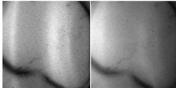
Figure 5. FCT in reflection mode for bone with differing layers of soft tissue, 0 mm (left) and 6 mm (right).
