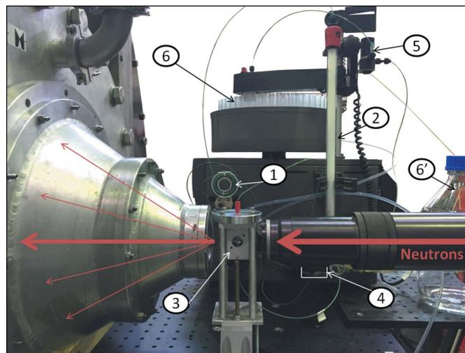
**Figure 1** Setup of *in situ* chromatography SANS. The sample is manually injected into the loop (1), then it passes through the size exclusion column (2), the SANS sample cell (3), the UV-visible spectrophotometer (4) and the valve (5), which directs it either to the fraction collector (6) or to the waste container (6').
