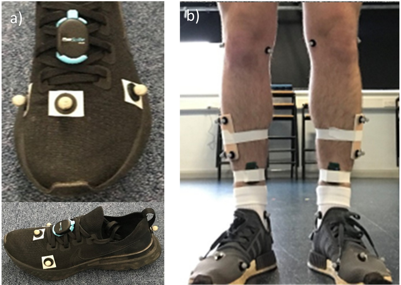
Fig 1. Marker and equipment placement on a) Participant footwear and b) lower limbs.
