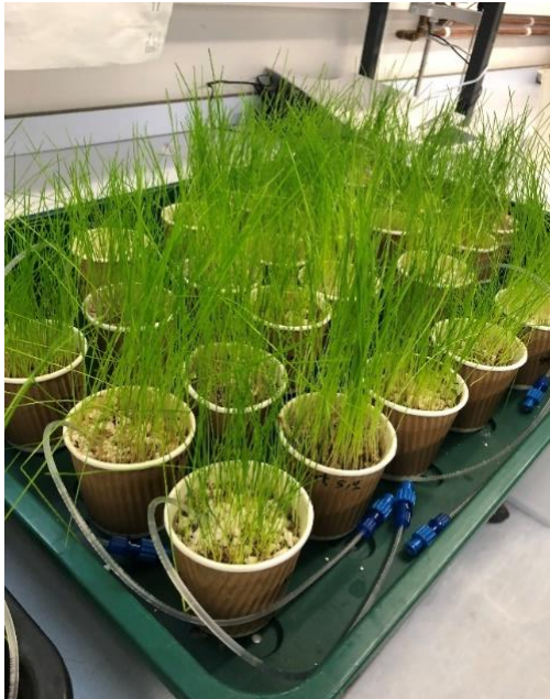
Supplementary Figure S1. Remediation trial setup illustrating pots equipped with rhizon soil porewater samplers (Rhizon Flex, Rhizosphere Research Products, The Netherlands) and plant growth 20 days after sowing.
